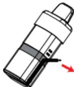
b. Remove the silicone shim between the pod and the container.
