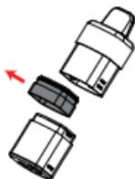
c. Install the pod to the container, and make sure they are firmly and properly connected to avoid leakage.
